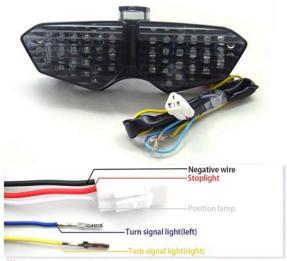
Tips: This is a multifunctional integrated taillights, including turn signal function. If you already have your own turn signal lights, or the laws of your country does not allow the use of the turn signal function of this taillight, it's also ok. It does not affect the operation of the taillights, Please feel free to contact us if any question.
